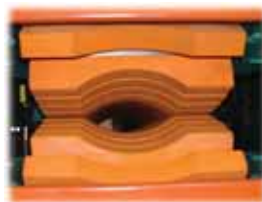
Custom-profiled cleats for solid or thick-wall hollow rods
