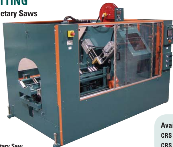
Planetary Saw CRS 6-18 (20 in. maximum O.D.)
