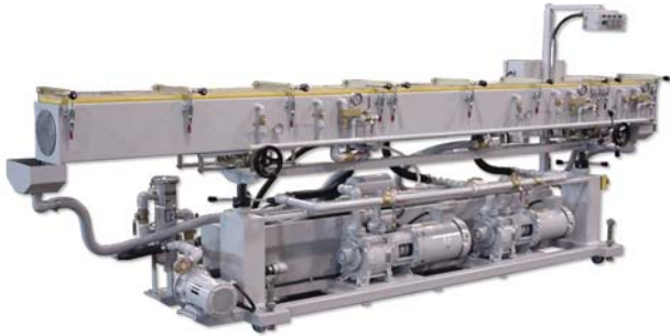
CVS 10-14 with water recirculation system
