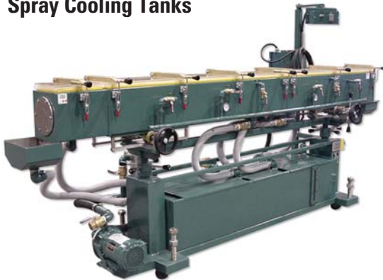
CVS 10-10 with water recirculation system
