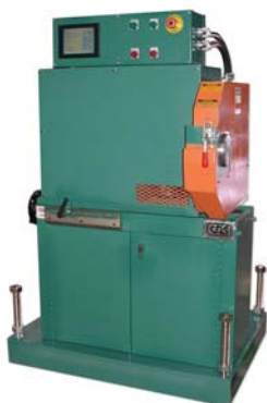
Servo Fly-knife Cutter CSFK 4.5 (4.7 in. maximum O.D.)
