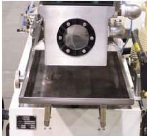
Pan Covers Length of the Tank for Maximum Coverage
